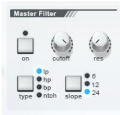
The Master Filter is applied to the entire output signal and is typically used for filter-fades where the cutoff is slowly increased or decreased during intros or breaks.
