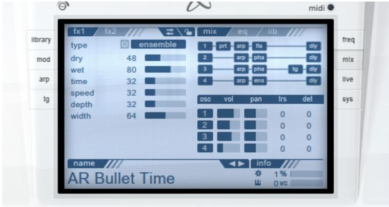
The left column of this page is used for controlling the two master effects. You can toggle between the two effect slots by clicking on their title. The two-arrow-symbol swaps the two effect slots with each other.
