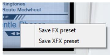
The browser displays the FX names with a category prefix. You don't need to edit them manually. The prefix is added automatically during save and removed during load.
